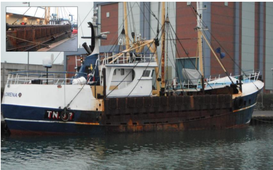
Plate 4 Over 15 m UK vessel converted from beam trawler to scallop dredger (BMM, 2016)
