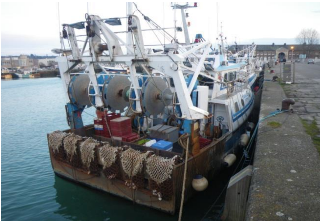
Plate 7 A Multi-purpose French fishing vessel operating scallop dredges from the stern (BMM)
